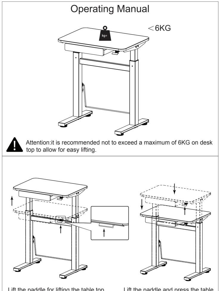
Lift the paddle for lifting the table top.
